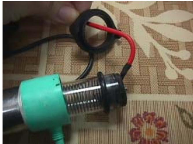
5. Clean the glass by soft cloth or tissue ( When Inner has green oxidize powder it's normal condition of chlorine chemical composition. Will Not effect the ozone output)
